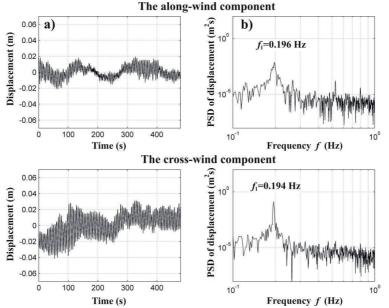
Fig. 19. a) The response of the TV Tower head at the level of H = 157 m (along and cross-wind components) start: 29/04//2011 – 12:02:00, interval 480 s, baseline 502 – 1202, b) Power spectral densities for both components
