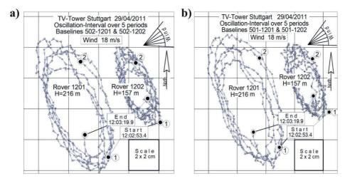
Fig. 20. Dynamical components of the wind response on the top of steel antenna mast and the TV Tower head, five vibration loops
