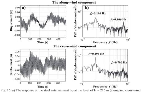
components), start: 29/04//2011 - 12:02:00, interval 480 s, baseline 501 - 1201, b) Power spectral densities for both components
