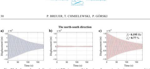
Fig. 23. In the north-south direction: (a) RD signature, (b) function of approximation inaccuracy, and (c) approximating function with an obtained damping ratio value
