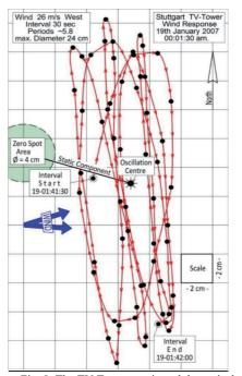
Fig. 8. The TV Tower, static and dynamical components of the wind response on the horizontal plane, 30 s detail, 01:41:20 a.m., a west wind of 26 m/s
