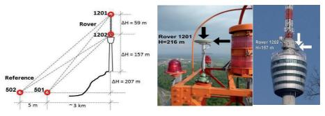
Fig. 10. Sketch for the arrangements of base lines with Reference and Rover receivers
